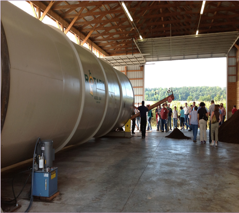
Figure 6-13. Rotating drum for carcass composting
