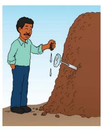
accurately weighing a representative sample of material before and after driving off moisture in an oven at 220°F (104°C) for 24 hours.
