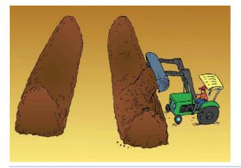
to be pulled by the tractor or loader. Other sidemounted units must be attached to a tractor and run through the power take-off (PTO). Side-mounted units turn half the windrow at a time, which means two passes must be made to turn each windrow. Side-mounted units require more space between the windrows than straddle units.
