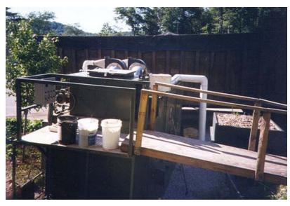
In-vessel composting unit with biofilter.
